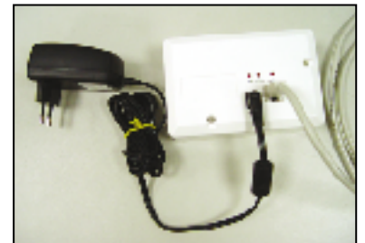
8. Use power adapter 5Vdc to power on, and connect the patch cord with RJ45 modular port.
