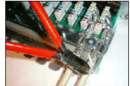
7. Thread the cable tie and cut the cable tie. Please do not use too much force to deform the cable.
