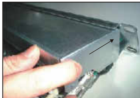
9. First, insert the cover front side into the panel hood.
